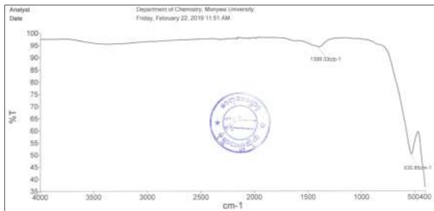
**Figure 4** FT IR spectrum of MF2 nanoparticles
