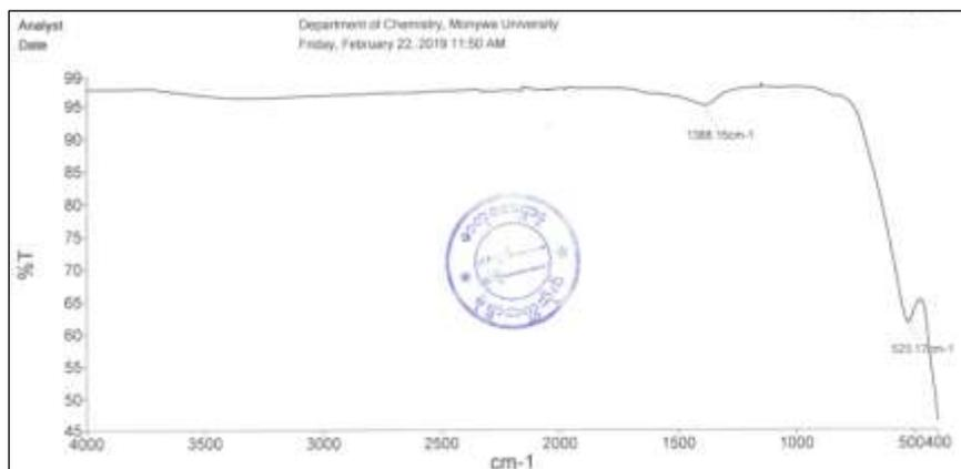
**Figure 3** FT IR spectrum of MF1 nanoparticles
