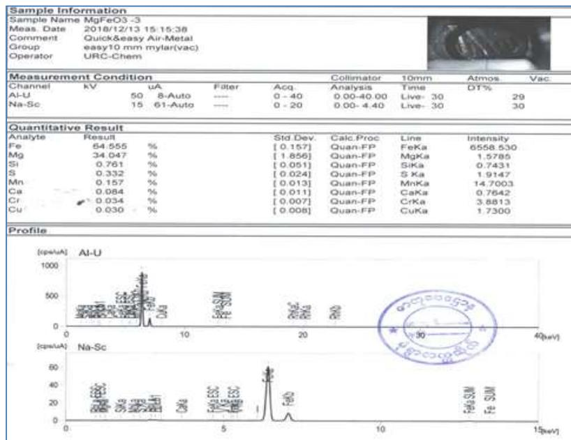
**Figure 1** EDXRF spectrum of MF1 nanoparticles
